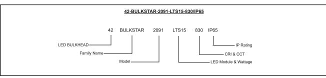
LED BULKHEAD BULKSTAR-2091-LTS15-830/IP65
