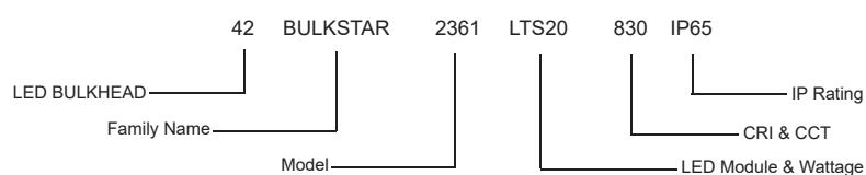
LED BULKHEAD BULKSTAR-2361-LTS20-830/IP65
